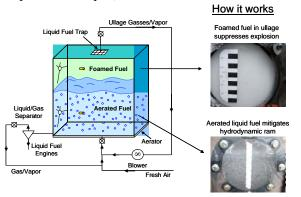
The two components of FuelShield<sup>TM</sup> (bubbles and foam) can be implemented separately or in combination with a synergistic effect. The system is designed to interface with commercial off-the-shelf equipment currently used in aircraft fuel systems.
