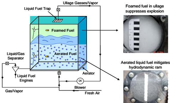
The two components of FuelShield™ (bubbles and foam) can be implemented separately or in combination with a synergistic effect. The system is designed to interface with commercial off-the-shelf equipment currently used in aircraft fuel systems.
