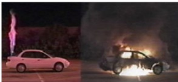
Fires from intentionally ignited hydrogen (left) v. gasoline (right) fuel tanks
